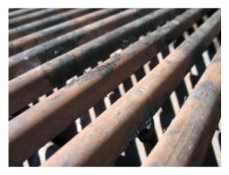
Of interest relative to the case study is that the two cleaners used by the Insured both contained "oxalic acid". This substance functions as a derusting agent by preferentially forming an "oxalate" with rusted iron, displacing ("precipitating") the rust and exposing the underlying bare metal. The use of this substance, followed by abrasion, allows the re-formation of a passivated, corrosion resistance surface on the stainless steel.
